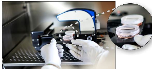
Figure 3: HoloMonitor ® M4 time-lapse cytometer with a motorized stage operating inside a cell incubator. To avoid condensation and surface vibrations a special lid was developed, which is partly immersed into the cell culture media (insert). Approximately 100 HoloMonitor units are currently in operation in cell laboratories around the world.
